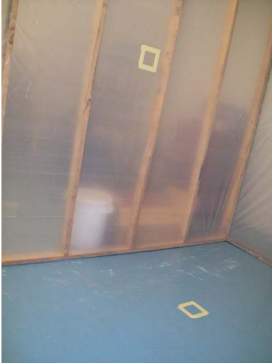
Swab sample locations in the temporary testing room
